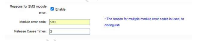
Module error code: When the error code is returned for the specified number of times during the sending of the SMS, the SIM will be locked!
