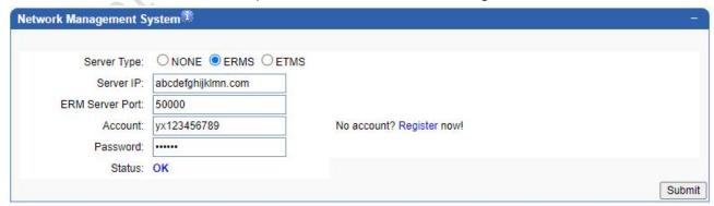
Remote Management is used to manage the GoIP Gateways located in other physical locations. Network must be available for the gateway to communicate with ERMS or ETMS Server, When the
