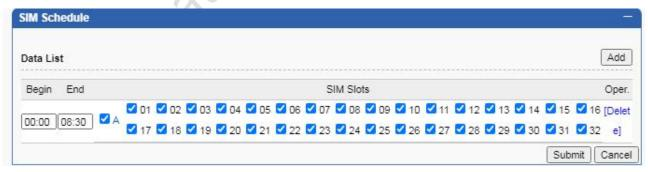
This function is used to set the SIM card usage policy, for example, As shown, it means that these SIM cards will be used between time: 00:00-8:30.
