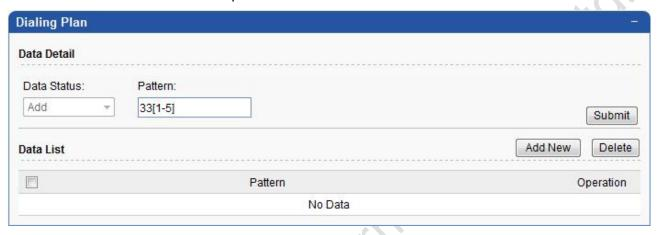
Dial Plan is a string which specifies digits and length of the digits of the dialed number. Generally, the pound sign # is used as the termination of number input for dialing. However, if patterns are specified and system detects the dialed number matches any of the patterns, it will stop collecting input and send out the collected number to dial even though no pound sign is encountered.
