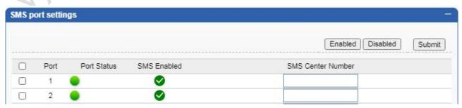
This setting can enable or disable the SMS function of the port, and set the SMS center number
