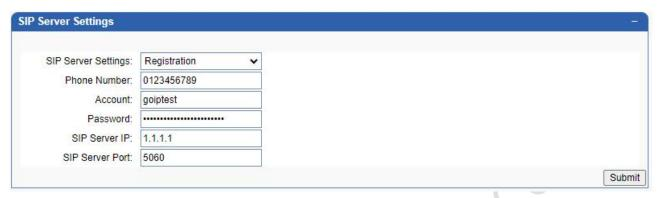
SIP Server Settings is for SIP communication with IP network. Fields are specified as following:
