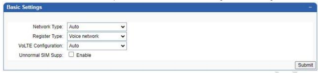
It's for choosing the frequency(Auto/2G/3G/4G) band and whether register type(Voice/Data), VoLTE enabled or not(Auto/Disabled/Forced). When the gateway can't detect the SIM and you sure the install SIM is right, we need to enable Unnormal SIM Support.
