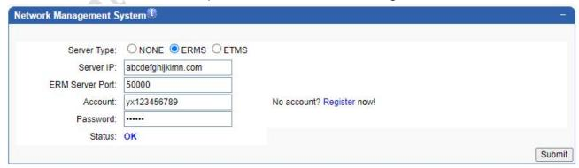
Remote Management is used to manage the MoIP Gateways located in other physical locations. Network must be available for the gateway to communicate with ERMS or ETMS Server, When the
