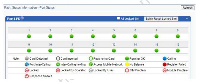
LED A/B/C/D(.01-.16) displays in accordance with the lights on the front board of MoIP Gateway. Port 1 to 4/8/16/32/64 relate to the physical port of MoIP Gateway. The following table shows the relationship between LED color and port status.( When registering a card, the description of the card may not be displayed in real time. Please refer to the information displayed on the icon)
