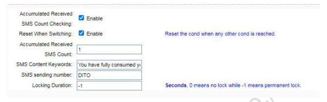
This function locks the SIP card after receiving the text message with the specified content sent by the specified number, for example, lock the SIM card according to the prompt message of insufficient balance!
