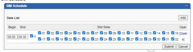
This function is used to set the SIM card usage policy, for example, As shown, it means that these SIM cards will be used between time: 00:00-8:30.
