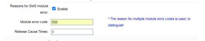
Module error code: When the error code is returned for the specified number of times during the sending of the SMS, the SIM will be locked!
