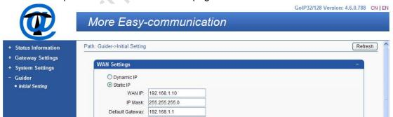
WAN port is to connect to switch or route then you can use PC that on the same LAN network to login. There's three types of wan connect.
